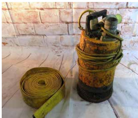
The Ponstar (to use the correct name; typically known as Pornstar by us) pumps used at Jenga Pot, with the accompanying 2-inch diameter lay-flat pipe. We have three of these in-situ at the time of writing, one for each of the three sumps.
