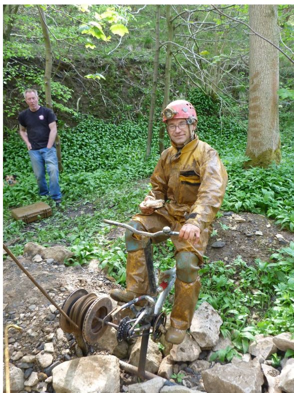
Richard 'Sparky' Edwards operating the remarkably effective Jenga winch 'bike', installed Jan 2013, which made hauling buckets faster and easier. Photo by Gary Douthwaite.
